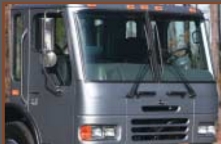
Two-piece windshield with optional side and rear window options provide for up to 273° of visibility to all corners of the cab
