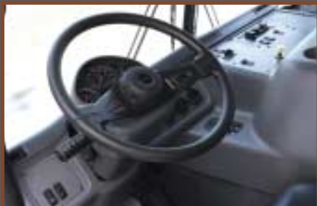
Dash-mounted steering column that tilts and telescopes with all critical gauges
